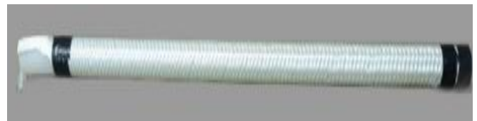
Fig. 2 Produced tubular braids
