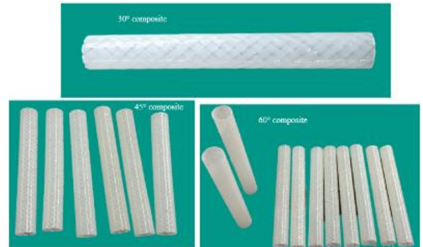
Fig. 9 2D braided composite cylinders
