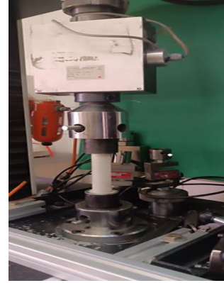
Fig. 12 Braided composite cylinder under tension
