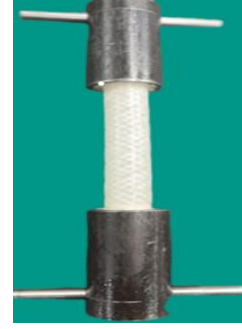
Fig. 11 Final prepared specimen for the tensile test
