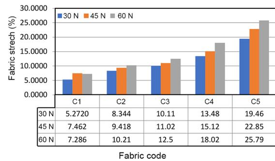
Fig. 5. Stretchability of denim fabrics at different spandex percentage.
