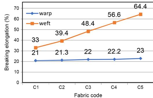
Fig. 3. Breaking elongation of denim fabrics at different spandex percentage.
