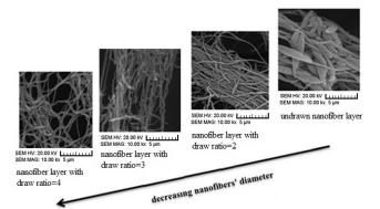
Fig. 3. Deformation of dispersed phase with increase in draw ratio.
