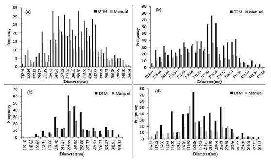
Fig. 10. Diameter distribution of nanofibers produced from blend fibers, obtained from manual method and FCM- DTM; a) undrawn, b) with draw ratio of 2, c) with draw ratio of 3, d) with draw ratio of 4.
