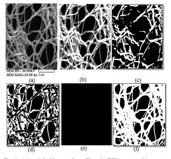
Fig. 4. a) An original image of nanofibers, b) FCM segmented image, c) FCM segmented layer1, d) FCM segmented layer 2, e) FCM segmented layer 3, f) thresholding image obtained from adding c and d.
