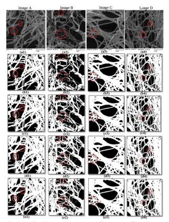
Fig. 7. Nanofiber images: A) undrawn nanofiber , B) nanofiber with draw ratio of 2, C) nanofiber with draw ratio of 3, D) nanofiber with draw ratio of 4. (a1-a4): original images, (b1-b4): Global thresholding, (c1-c4): Local thresholding, (d1-d4): K-means thresholding, (e1-e4): FCM thresholding.
