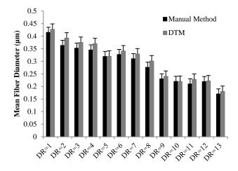
Fig. 11. The mean diameter distribution of fibers in different drawing ratios calculated by manual method and DTM.
