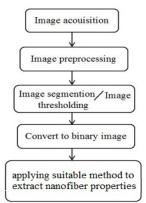
Fig. 1. Flowchart of determining nanofiber properties using image processing.
