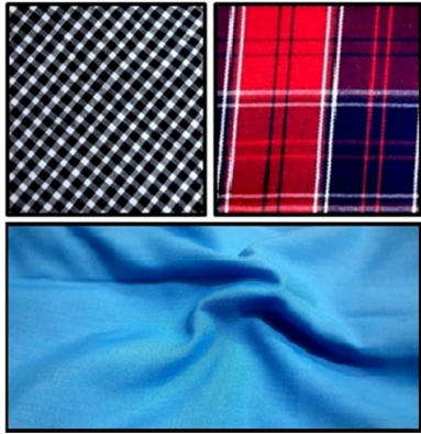
Fig. 1. Plain, twill and satin fabric used in this research.
