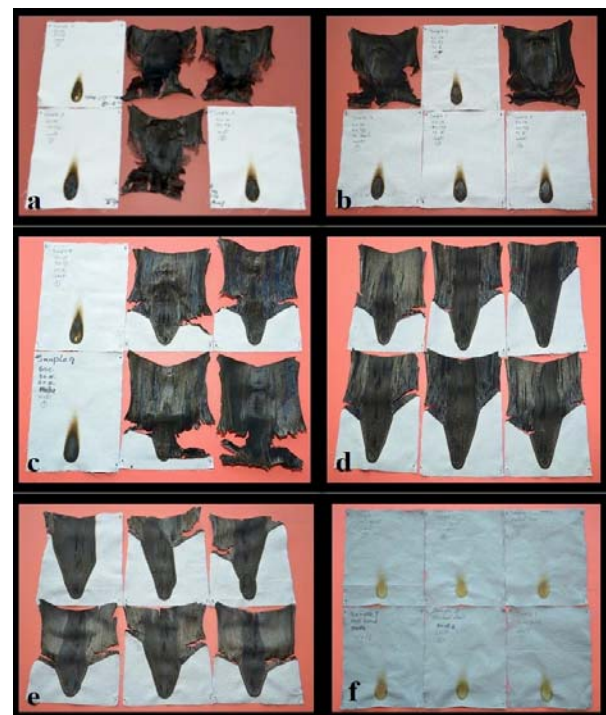
Fig. 8. Photos of cotton/nylon-Kermel blended fabric samples exposed to vertical fire: a) Sample1 (Co50/Ny50), b) Sample2(Co50/Ny40/K10), c) Sample 3 (Co50/Ny30/K20), d) Sample 4 (Co50/Ny20/K30), e) Sample 5 (Co50/Ny10/K40), f) Sample 6 (K100).
