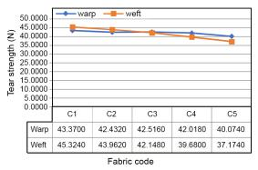
Fig. 4. Tear strength of denim fabrics at different spandex percentage.
