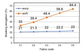
Fig. 3. Breaking elongation of denim fabrics at different spandex percentage.
