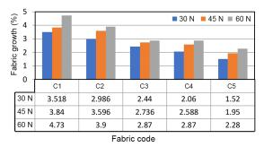
Fig. 6. Fabric growth of denim fabrics at different spandex percentage.
