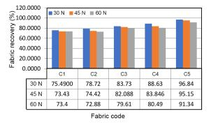
Fig. 7. Fabric recovery of denim fabrics at different spandex percentage.
