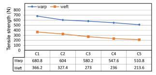
Fig. 2. Tensile strength of denim fabrics at different spandex percentage.
