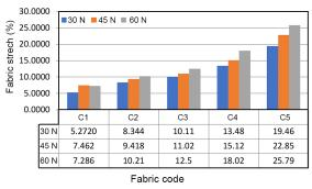
Fig. 5. Stretchability of denim fabrics at different spandex percentage.
