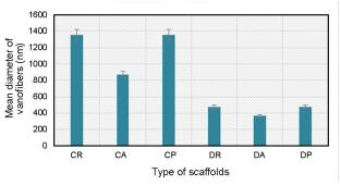
Fig. 2. Mean diameter of non-treated, structurally-modified, and plasma-treated nanofibers in two groups.
