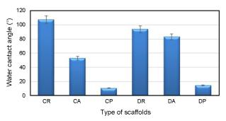
Fig. 6. Water contact angle values for the non-treated, structurallymodified, and plasma-treated scaffolds in two groups; there is no significant difference between the hydrophilicity of the two groups of scaffolds (C and D).
