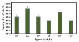
Fig. 4. Porosity of non-treated, structurally-modified, and plasma-treated scaffolds in two groups; there is significant difference between the porosities of two groups of scaffolds (C and D).
