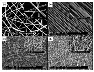
Fig. 1. SEM micrographs of scaffolds: (a) CR, (b) CA, (c) DR, and (d) DA (magnifications: 1000x, 5000x).
