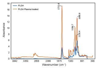
Fig. 5. ATIR-FTIR spectra for non-treated PLGA and argon plasma treated PLGA.
